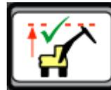
The system will ask if you want to enter the maximum height limit with the keyboard. Pressing “YES” will bring up a keyboard screen. Enter the height in metres and press OK. [Pressing exit without entering data will switch off the limit].
